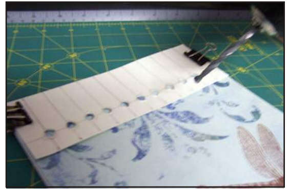
Affix template and drill holes at cross sections
